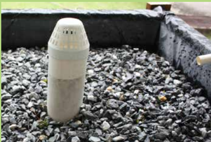
When the water in the grow-bed rises to a certain level, the bell syphon automatically opens a valve to flush the water back into the fish tank. (Photo credit: Rachel Laramée (RL))
